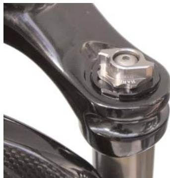
Turning knob for adjusting the MEKS Carbon AC pre-load.
