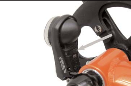
You switch on the hub generator light system with the integrated switch at the front light.
