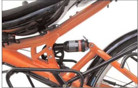
Air Shock DT-Swiss XMI80. The damping is adjusted with the red wheel at the rear end. The rear shock must be mounted with the lever on the rear end facing upwards to avoid crashing into the swing arm.
