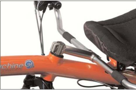
The handlebars are connected to the front fork by an A-Head stem. The two bolts on the side of the stem clamp it on the steerer tube of the front fork.
